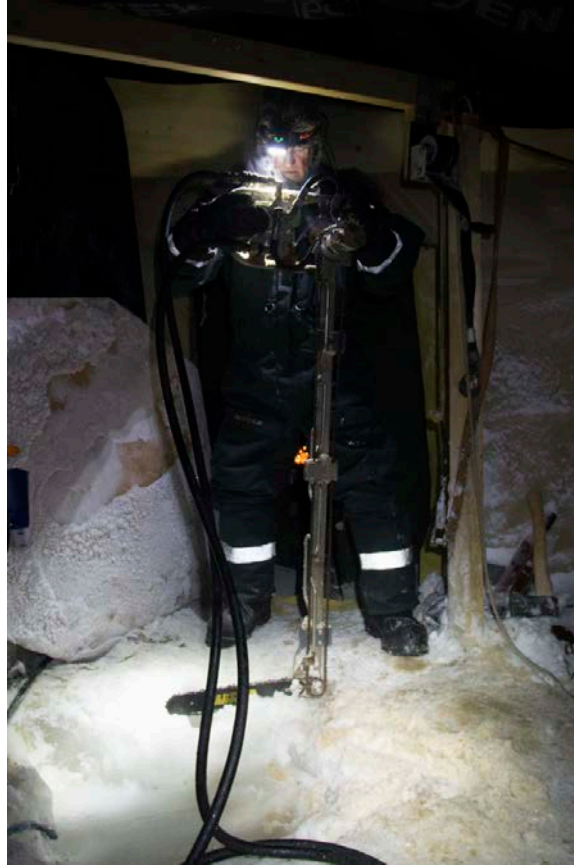
Fig. 2. The new hydraulic chain saw invented for making vertical cuts in the ice. This prototype made from junk yard resources works well.
